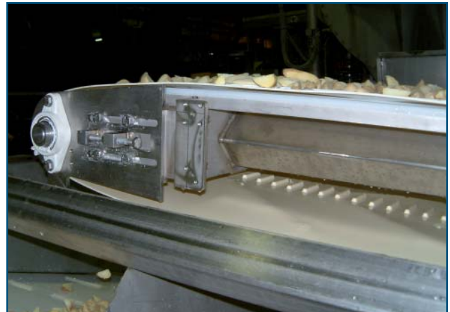
FHW-3-SD Integral teeth function as a guide for the belt
