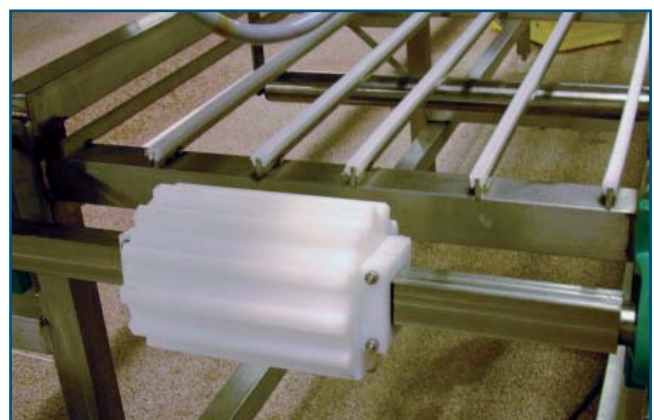
Figure 5: SuperDrive™ drive pulley with typical square shaft
