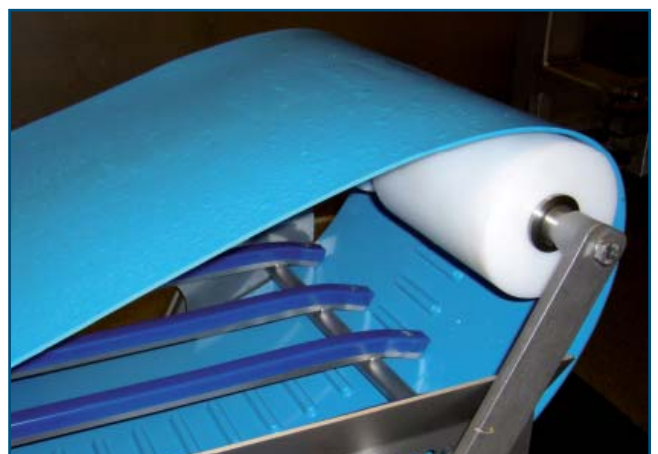
FHB-3-SD: Shows the tail pulley and slidebed
