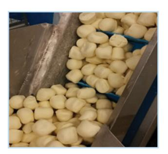
Other Dairy Products: Products like powdered milk are often repacked into consumer packaging and the prevention of loose fibres from ply belts entering the food flow is a major concern. Volta Metal Detectable (MD) belting can give additional security in some cases.
