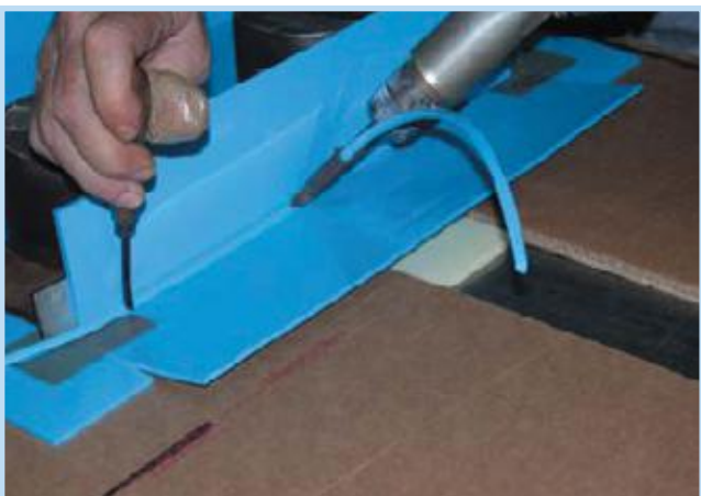
Electrode welding of cleats
