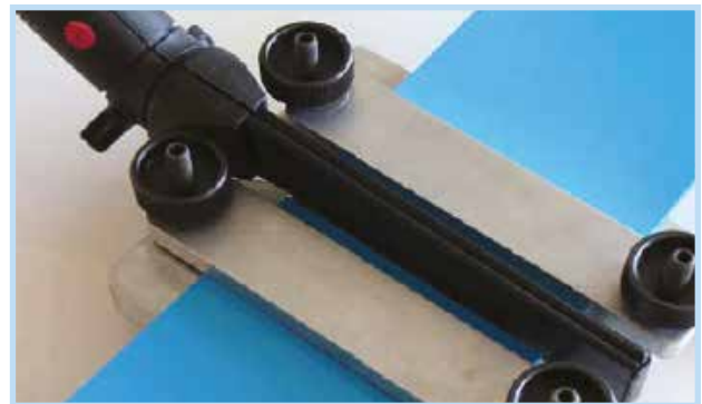
Welding narrow flat belts with Pliers P-200
