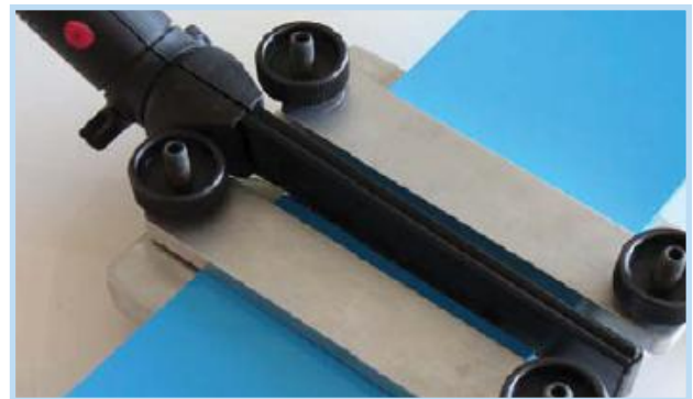
Welding narrow flat belts with Pliers P-200
