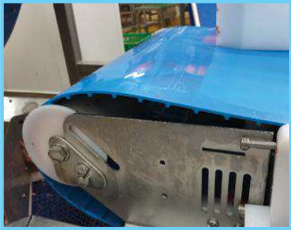
UHMW roundel mounted on pulley
