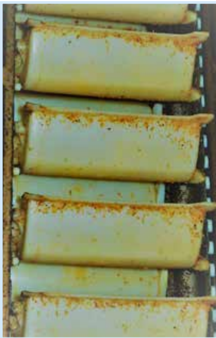
Open chain contaminated by food soil
