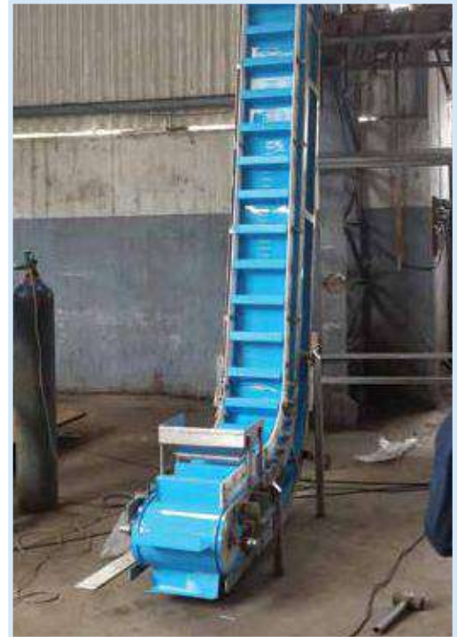
Fixed conveyor side wall
