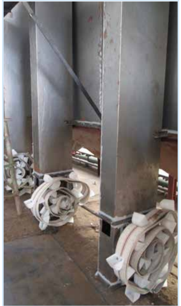
A battery of friction driven bucket elevators used in elevating tea leaves
