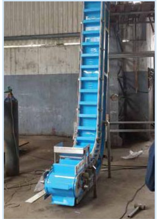
Fixed conveyor side wall
