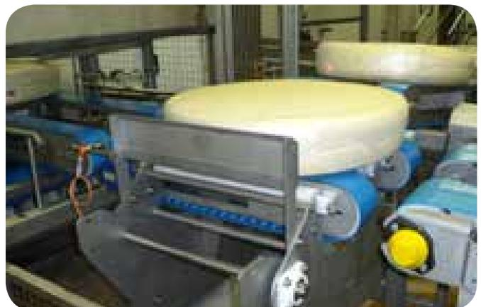
**Secondary Processing** – a significant percentage of cheese production goes through secondary processing, whether as reworked cheese mass or sliced for packs or grated for further use in products such as pizzas. This necessitates transporting on additional conveying systems where hygiene becomes critical as the product is exposed yet again to belting surfaces.
