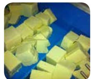
**Deep Freeze Applications:** The Volta Low Temperature (LT) belt material is unique in its ability to work well in temperatures well below zero for transporting frozen cheese in grated or block form. The LT material does not stiffen and can be used on relatively small pulley diameters as well as not damaging from the action of frozen product.
