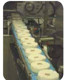
**Hard Cheese:** Volta's homogeneous flat belt material will not absorb water and oils and has no ply. Ply is prone to soak up liquids thereby developing high concentrations of bacteria and causing cracks to form in the laminated surface. Volta smooth surface belts can be scraped with no resulting damage to welded joints and no danger of grooving. Further fabrications such as flights and side walls for containment make this system adaptable to elevators and even swan-neck conveyors.
