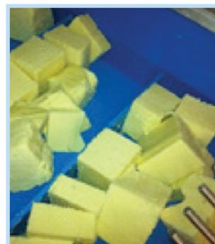
✓ **Deep Freeze Applications:** The Volta Low Temperature (LT) belt material is unique in its ability to work well in temperatures well below zero for transporting frozen cheese in grated or block form. The LT material does not stiffen and can be used on relatively small pulley diameter. It will not be damaged by the abrasion of the frozen product.
