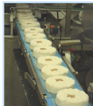
✓ **Hard Cheese:** Volta's homogeneous flat belt material will not absorb water and oils and has no ply. Ply is prone to soak up liquids thereby developing high concentrations of bacteria and causing cracks to form in the laminated surface. Volta smooth surface belts can be scraped with no resulting damage to welded joints and no danger of grooving. Further fabrications such as flights and side walls for containment make this system adaptable to elevators and even swan-neck conveyors.
