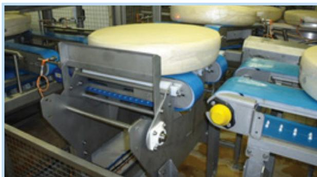
✓ **Secondary Processing -** a significant percentage of cheese production goes through secondary processing, whether as reworked cheese mass, sliced for packs or grated for further use in products such as pizzas. This necessitates transporting on additional conveying systems where hygiene becomes critical as the product is exposed yet again to belting surfaces.
