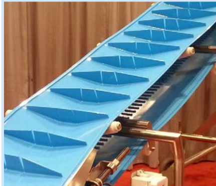
Special cleats on trough conveyor
