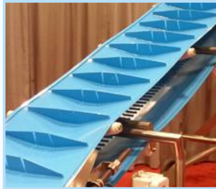
Special cleats on trough conveyor
