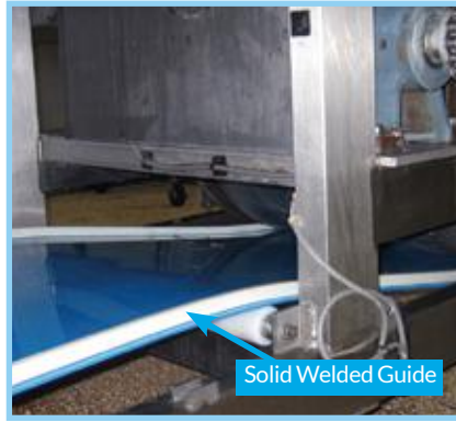
2. Two parallel guides on, or close to the belt edges on the underside of the belt; common in vegetable processing.
