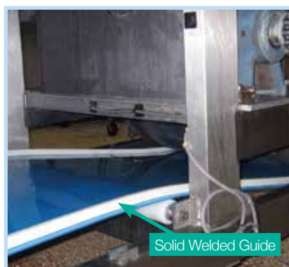
2. Two parallel guides on, or close to the belt edges on the underside of the belt used on wider belts; common in vegetable processing.
