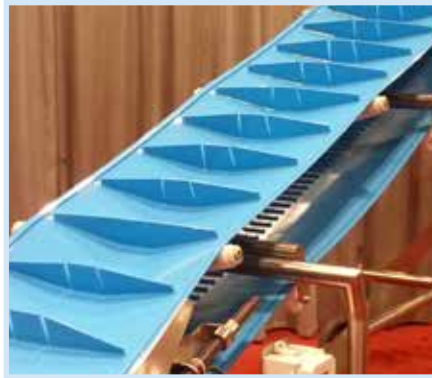
Special cleats on trough conveyor
