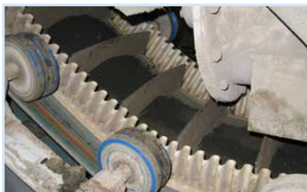
FRG-3 with thermo welded sidewalls and flights: CHEMICAL POWDER (RECYCLED SEWAGE)
