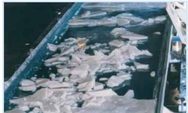
FZ-5: CONVEYING CAUSTIC SODA
