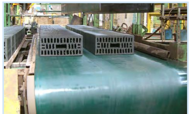
FRZ-4: HEAVY BRICK CONVEYING
