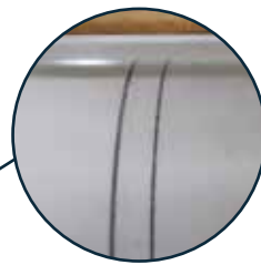
Damaged belt due to unsuitable Scraper
