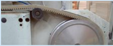
Edge Bander Belt Section: SP - 2C Quantity In Machine: 1
