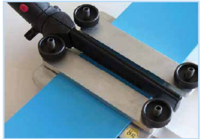
Welding narrow flat belts with Pliers P-200
